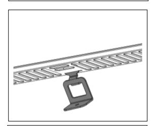
3.) Hook the Lower Bracket into the slit at the bottom of the heater.
