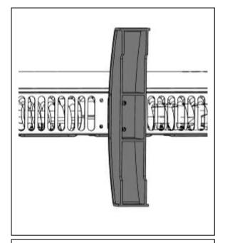
1.) Using the 12mm screws supplied, fit each foot as illustrated above.
