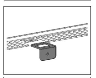
4.) Fix Lower Bracket into position using 30mm screw and wall plug. The heater is now ready to use.
