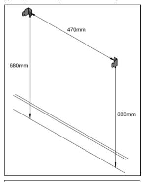
1.) Using the 30mm screws and wall plugs supplied fit the Upper Brackets, as illustrated above.
